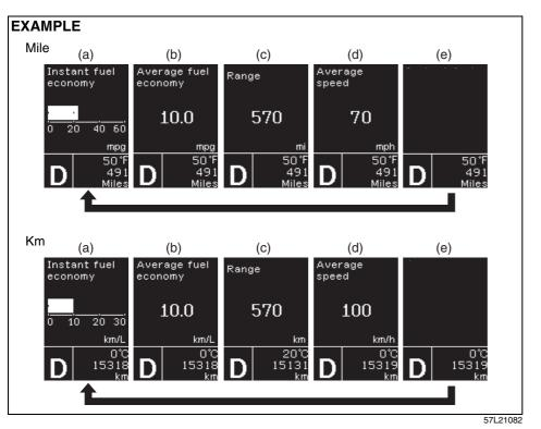
To switch the display indication, pull the DISP switch (2) quickly.
